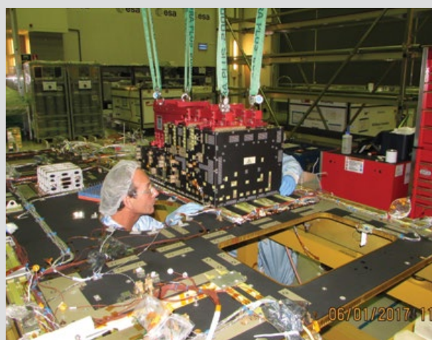
Reintegration of the second Power Processing Unit on the BepiColombo Mercury Transfer Module
