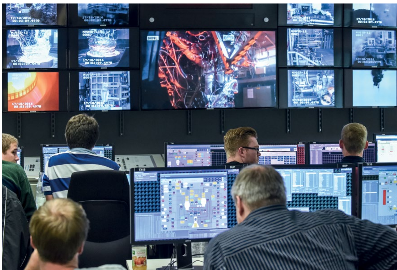
↑ During the test, cameras transmit what is happening in and around the test stand. The control room is a protected area (DLR)
